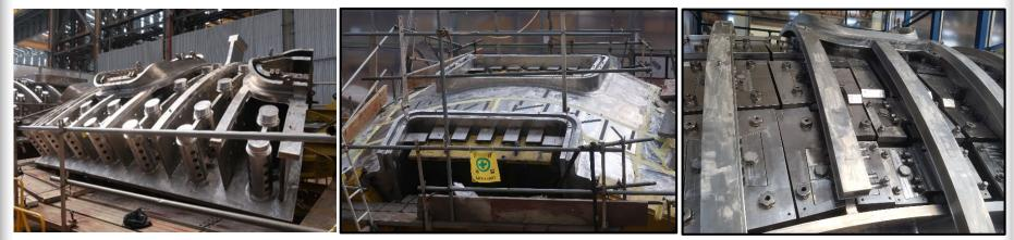
Poloidal Segment #2 (PS2): T-rib, Flexible Support Housing and In-Wall Shielding Support Rib Assembly Poloidal Segment #3 (PS3): Outer Shell Welding Assembly
